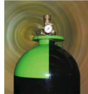
Extinguishant IG-541 is a colourless, odourless, electrically non-conductive gas with a density approximately the same as that of air. It is an inert gas mixture consisting nominally of 52% nitrogen, 40% argon and 8% carbon dioxide, with the following mixture specification (based on 8% carbon dioxide with tolerance of 3.5%).
